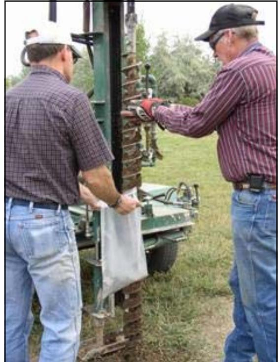
Design Engineer, Rex Stambaugh and State Engineering Geologist, Stan Mitchen drilled soils samples along the proposed flood wall to determine the water table and soil structure.
